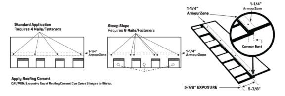
**STEP 9: INSTALL THE FIRST COURSE:** Start with a full length shingle applied flush with starter course at rake and eave. Use four nails per shingle placed as shown below. After the first shingle in the course is installed, continue with full length shingles to complete the first course, trimming the last shingle so that it matches the overhang of the starter course below.
