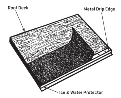
STEP 4: UNDERLAYMENT: Apply underlayment, either asphalt saturated felt or synthetic underlayment, such as IKO's Stormtite<sup>TM</sup>, in horizontal courses up the roof with 2" side laps and 4" end laps. Trim the sheet to fit the final course at the peak. One layer of asphalt saturated felt (or equivalent) is required over the entire deck to qualify for an ASTM E108 Class A fire rating or which
