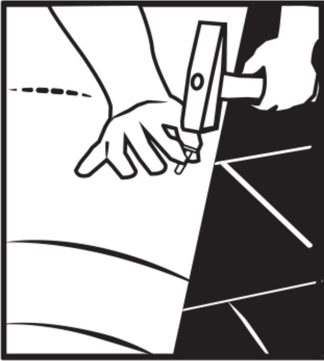
**FASTENERS:** Nails must be 11 or 12-gauge roofing nails, corrosion-resistant, with at least 3/8" heads, and at least 1" long. For decks 3/4" thick or thicker, nails must go at least 3/4" into the deck. On thinner decks, nails must go at least 1/8" through the deck.
