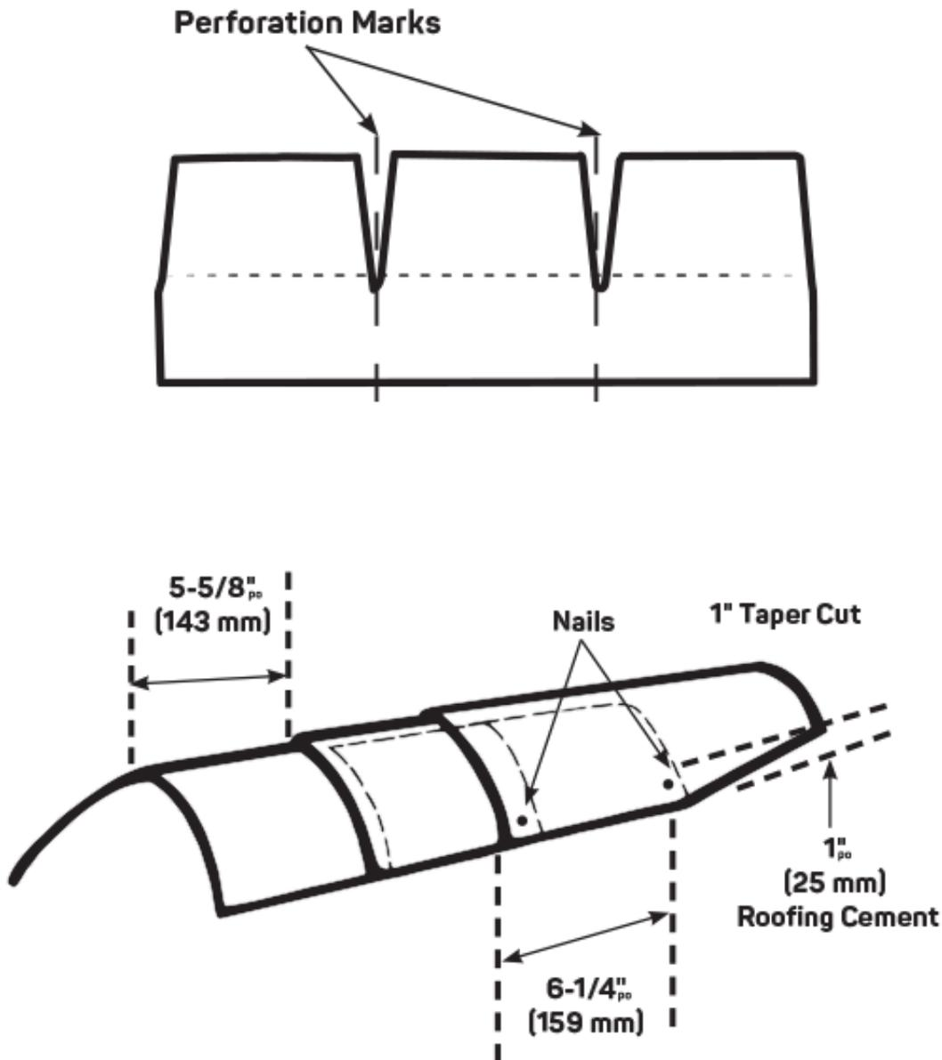
**STEP 12: BEND EACH PIECE OVER THE HIP OR RIDGE :** Nail 6-1/4" above the butt edge 1" in from each edge, exposing each piece 5-5/8".
