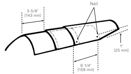
**Note:** To obtain a three-dimensional effect, (which is recommended, but not required), apply hip and ridge shingles double thickness by stacking two pieces on top of one another, the lower piece extending about 3/4" (19 mm) farther than the top piece.
